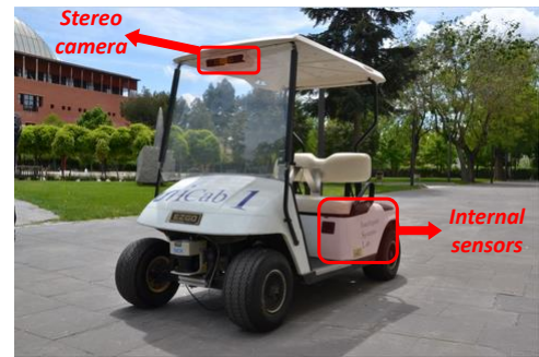
Fig. 13: Robotic vehicle of our case study used for assessing proprioceptive and exteroceptive models.
