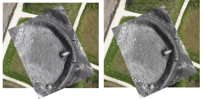
(c) Registered after homography of raw (distorted) images. (d) Registered after homography of undistorted images.
