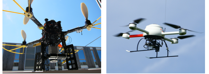
(a) AscTec Pelican drone with an FLIR Photon 640 thermal camera. (b) MD4-200 drone with an RGB camera.
