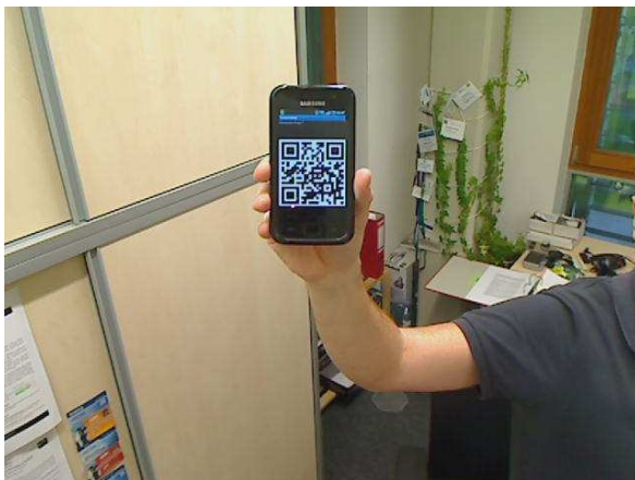
Fig. 8 A 2D barcode containing a visual attestation request as seen by the camera.
