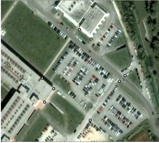
Fig. 13. Deployment of the cameras (black circles) on the monitored environment. Each camera is placed at height 14m.
