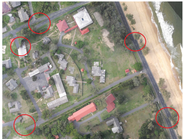
(c) Stitching disparities caused by inaccurate camera angle or position (red circles). [1].
