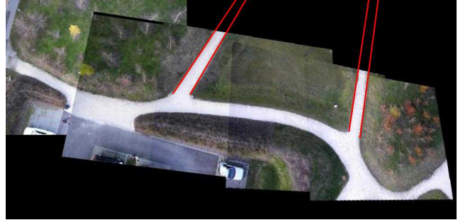
(a) Mosaicking five images using SURF features. The path borders (red lines) are supposed to be almost parallel. This type of error accumulates over multiple images if not compensated.
