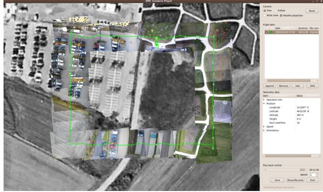
Figure 6. Screen shot of the GUI of our UAV system. The captured images are incrementally stitched over the—partially outdated—background image.
