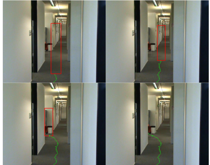
Fig. 4. A sequence of images showing the location of a tracked person as seen on the control station. Location information is transmitted via 802.15.4.
