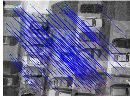
Figure 1: Overlapping image area with camera motion vectors
