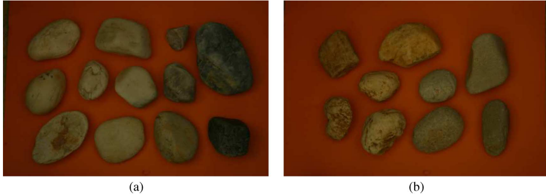
Fig. 15. Example materials for granulated material separation: (a) precious rubble (referred to class 1) and (b) worthless rubble (referred to class 2).
